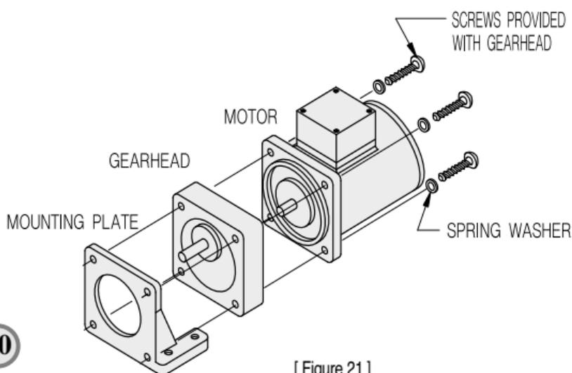
[Note] Secure all parts tightly by closing all gaps between the motor flange surface and mounting plate surface. Forced assembly of motor and gear head may cause erroneous noise and/or shorten the lifespan of the product.
