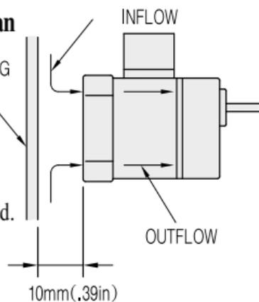
[Caution] Blocked cooling inlets shorten motor life and cause damages to the motor.
